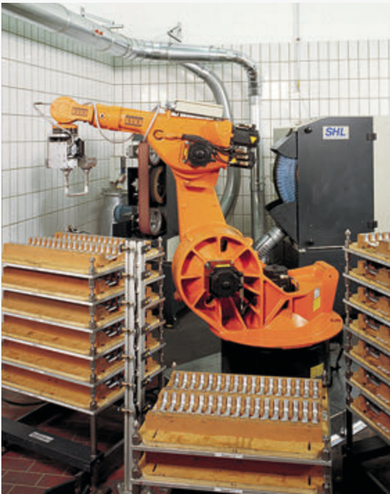
Roboter, Schleif- und Bürstanlage Robot, grinding and brushing machine
